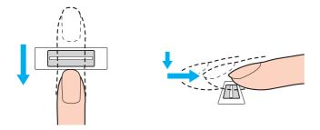
Keep your finger in contact with the fingerprint sensor while swiping.
